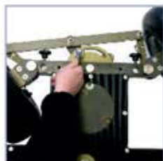
Steering transmission lock off
